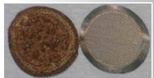
Left: Plugged fuel filter screen Right: Clean fuel filter screen
