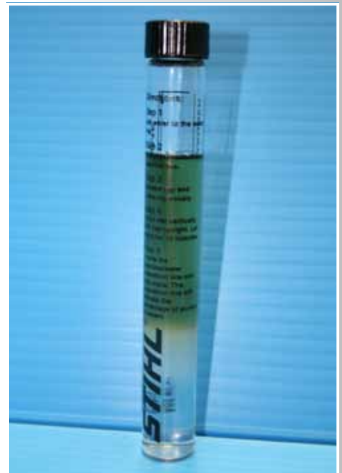
Water and ethanol (bottom layer) separated from gasoline (top layer)
