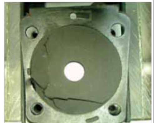
Damage to carburetor diaphragm
